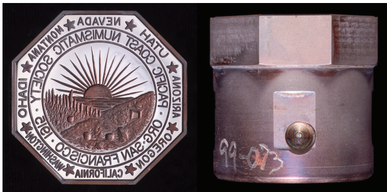
Figure 6: The PCNS 1975 replacement die created by Medallions Unlimited.
